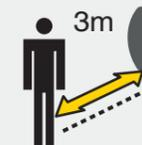
During inflation, stand in line with the tire tread minimum three meters away
