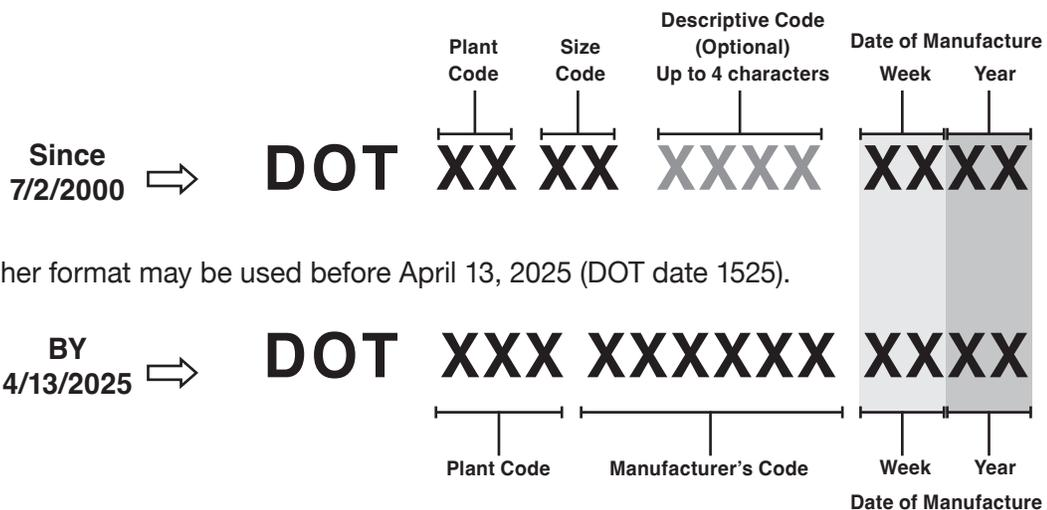
Note that the last portion of the TIN is changed—identifying the tire manufacture date using the same format for week and year. (For tires made before 7/2000, there is one digit for the year.)
