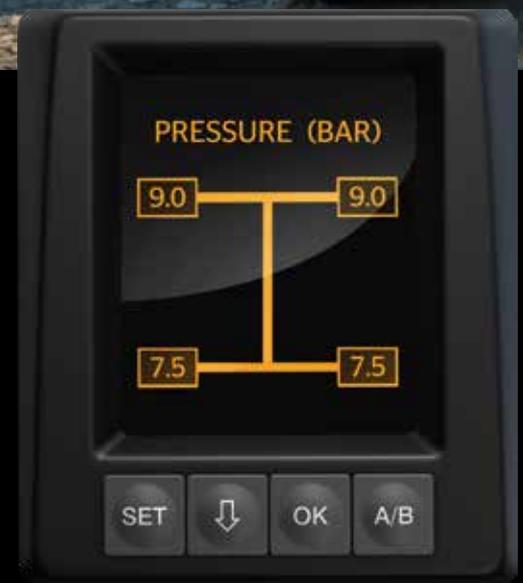
**ContiPressureCheck™ Integrated** allows OEMs and telematic providers to offer end users an easy solution for monitoring tyre pressure and temperature which will be integrated into their on-board (telematics) system.
