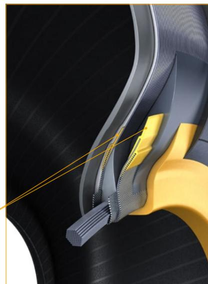
Edge protection component for very high resistance against crack propagation and mechanical stress
