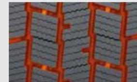
**4-Channel Pattern with Zig-Zag Grooves and Deep Full Depth Grooves**
