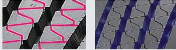
Combination of straight and zig-zag grooves provides better performance for traction and driving.
