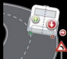
Load fluctuations due to centrifugal forces plus high centre of gravity, e.g. in bends
